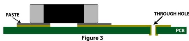
such as a via hole or wide trace, it will create a temperature difference ( $\Delta T$ ) on two sides of the component and cause tombstoning (Fig 3).
