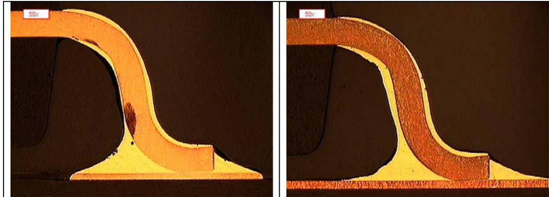
Fig 3. Vibration micrographs. Left: SAC305 TSOP. Right: Cobalt TSOP.
