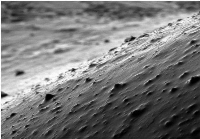
Fig. 7. Magnified solder joint showing no tin whiskers
