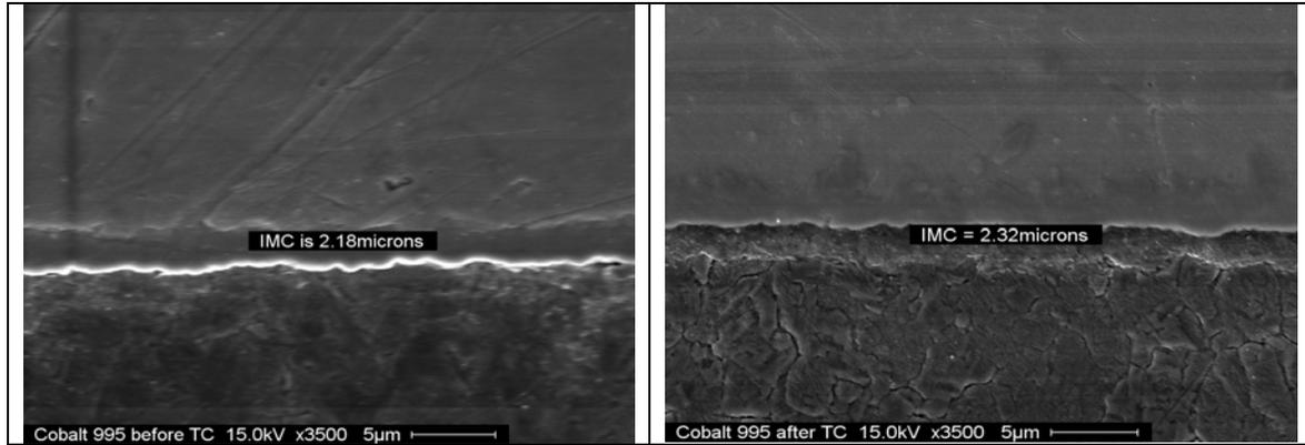
Fig. 4. Micrographs of inter-metallic layer. Left: cobalt enhanced alloy before thermal cycling.. Right: cobalt enhanced alloy after 1,000 cycles.
