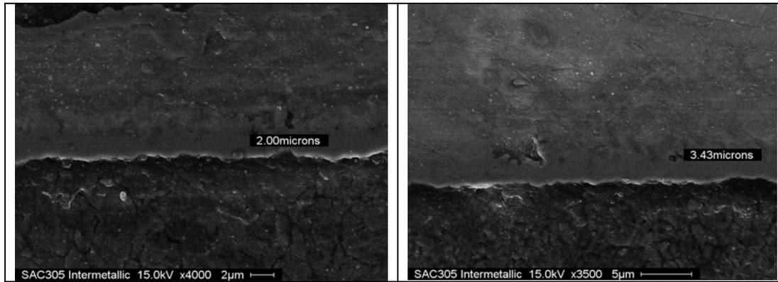
Fig. 5. Micrographs of inter-metallic layer. Left: SAC305 alloy before thermal cycling.. Right: SAC305 alloy after 1,000 cycles.
