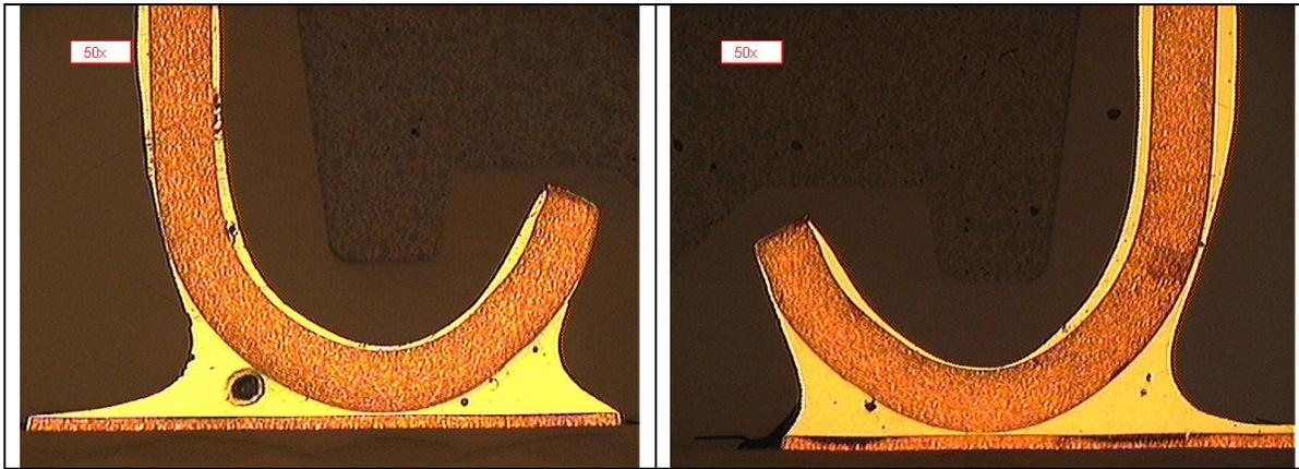
Fig. 1. Micrographs after thermal cycling. Left: SAC305 J-Lead. Right: Cobalt J-Lead.
