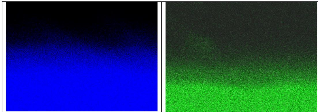
Fig. 6. X-ray map of copper diffusion in cobalt alloy (left) and SAC305 alloy (right).
