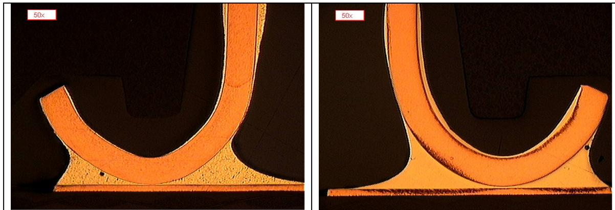
Fig. 2. Shock Test micrographs. Left: SAC305 J-Lead. Right: Cobalt J-Lead
