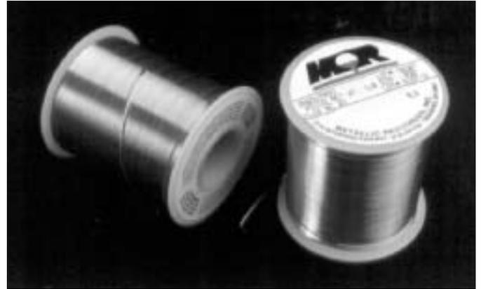
All water soluble fluxes tend to absorb moisture and some spattering is to be expected. Flux spattering can be minimized by applying the solder wire between the joint to be soldered and the soldering tip of the iron. Cored wire solder should not be directly applied to the tip of the soldering iron. After the re-work application, the flux residue on the board must be cleaned and removed with hot distilled or deionized water (140°F or 60°C minimum).
